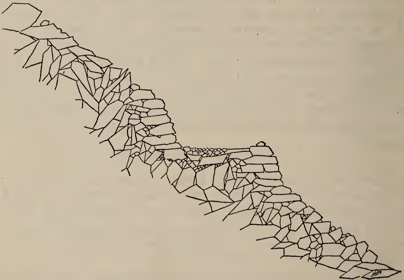
FIG. 12.—Retaining walls through rubble slides.
